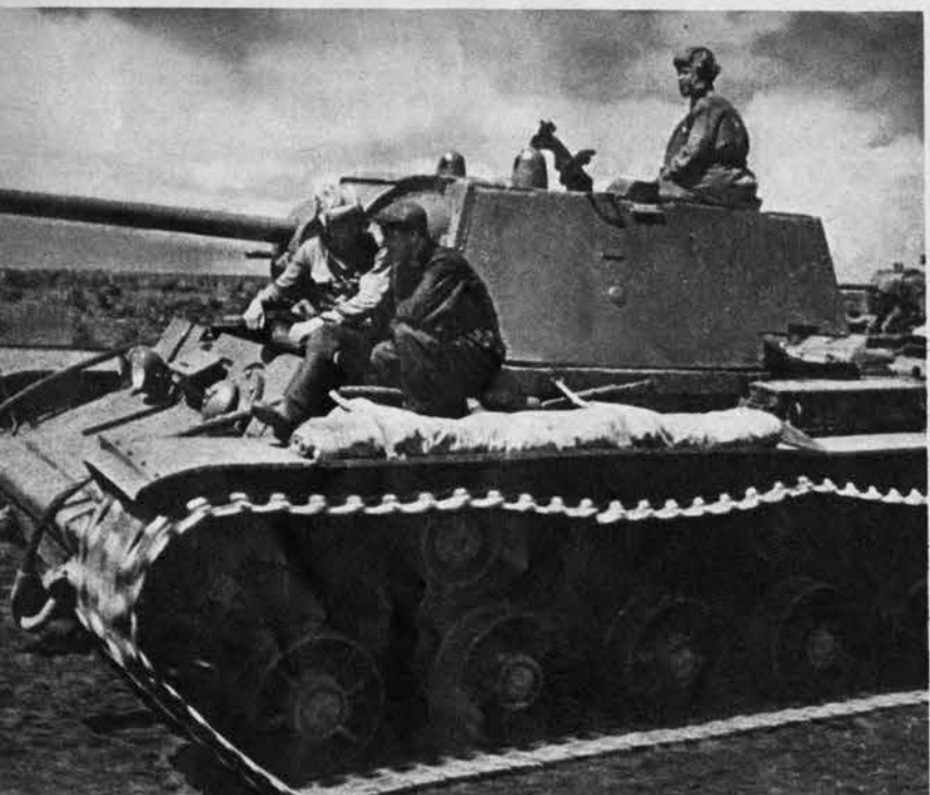
Russian KV-1 (above) and U. S. M-18 (below) have suspensions which loosely resemble Nazi PzKw's III and IV. KV-1 has six bogie wheels, three rollers; M-18 has five wheels, four rollers and a front drive.
